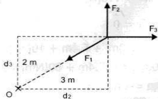
$$\begin{aligned}\tau_o &= \tau_{F1/o} + \tau_{F2/o} + \tau_{F3/o} \\ \tau_o &= F_2 \cdot d_2 + (-F_3 \cdot d_3) \\ \tau_o &= 5[\text{N}]3\text{m} - 12[\text{N}] \cdot 2\text{m} \\ \tau_o &= -9[\text{Nm}]\end{aligned}$$
